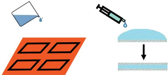
Deposition of Thin Polymer Film
