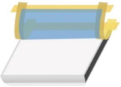
Delamination from Substrate
