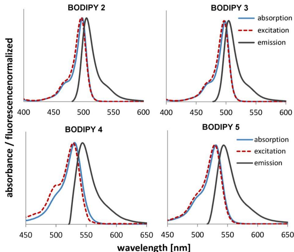
The long-wavelength absorption, excitation and emission bands for BODIPYs **2-5** in methanol.
