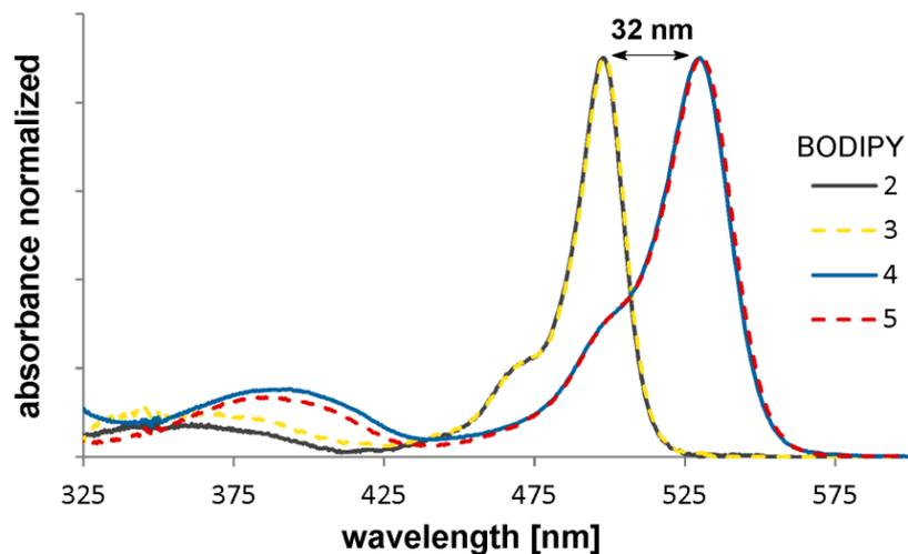
Maximum absorption ( $\lambda_{\max}$ ) and molar absorption coefficients ( $\log \epsilon$ ) for derivatives 2-5 in methanol
