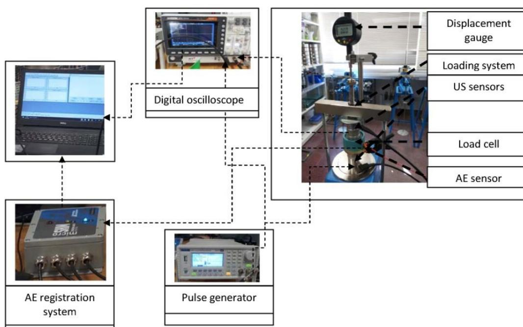
**Figure 1.** The setup of the US-AE-oedometer experiments.
