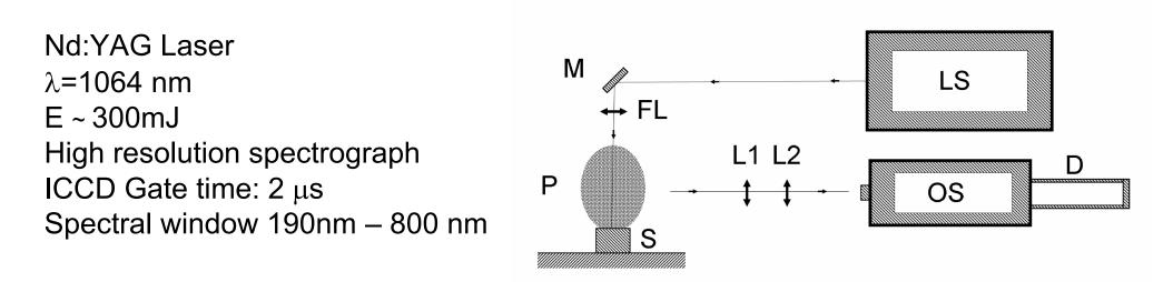
Schema of laser-induced breakdown spectroscopy (LIBS):
