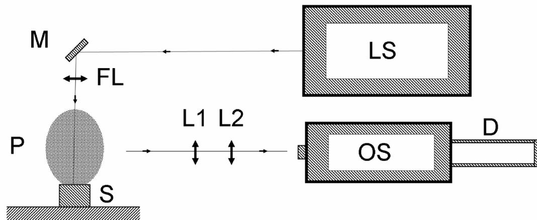
Schema of laser-induced breakdown spectroscopy (LIBS):
