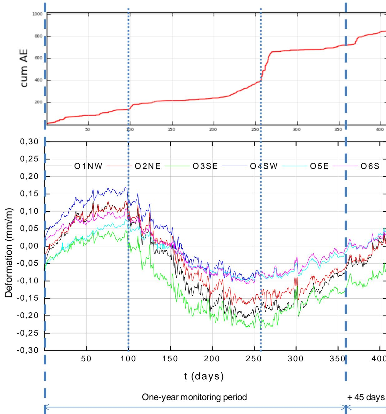
The comparison between the two diagrams shows that around the 100th day from the start of monitoring there is a significant increase in AE activity, also highlighted by a change in the strains growth.
