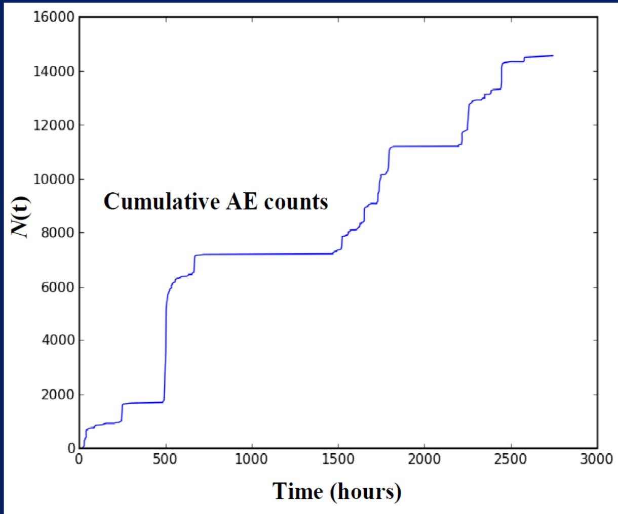
From the curve it can be seen that the masonry was undergoing a damage process.
