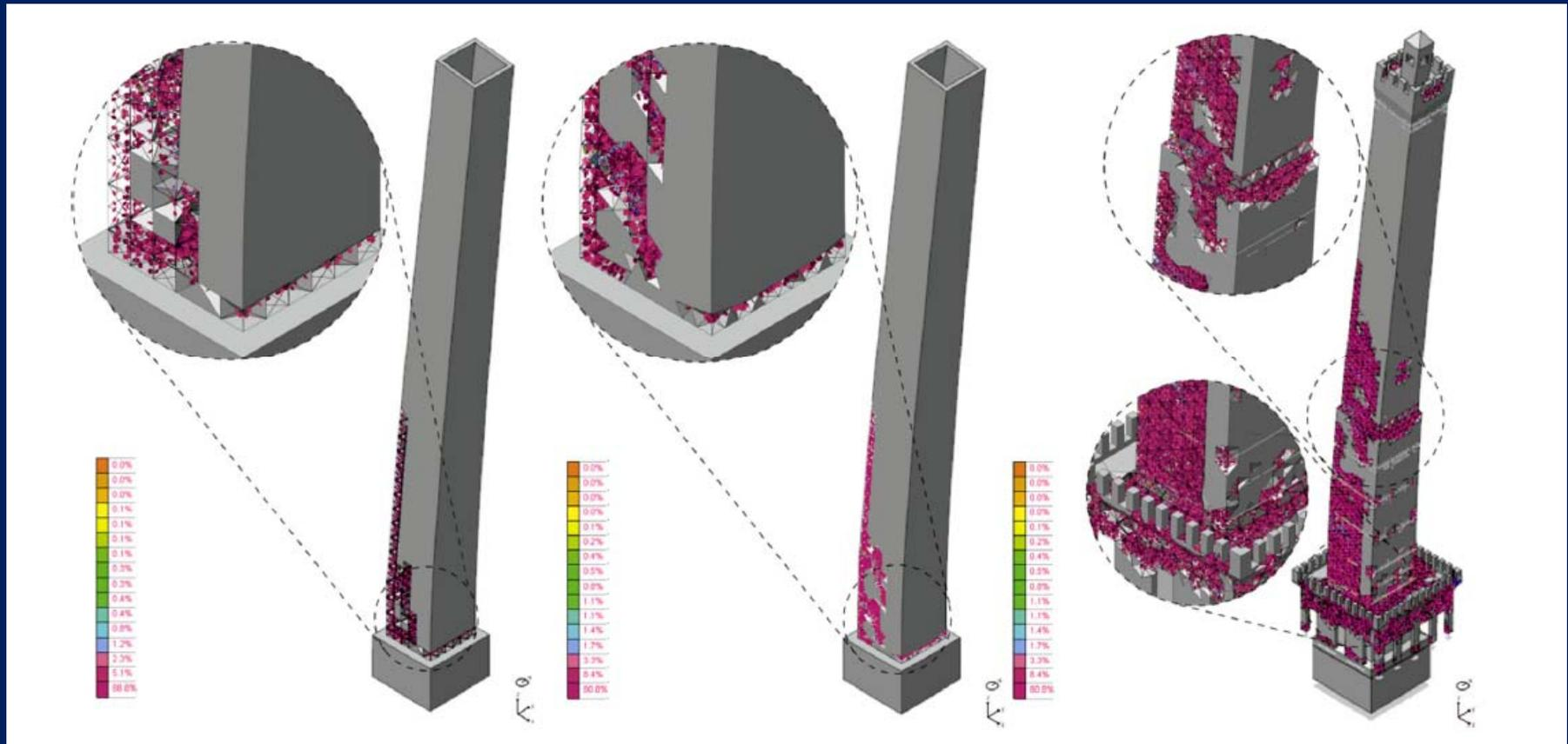
In the more complex model cracking energy distributes in a much realistic way compared to simplified models, since various discontinuities on the Tower have been modeled: openings, merlons, steeple, and so on.
