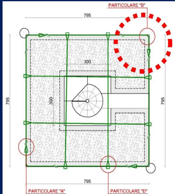
The AE transducers were applied to the north-east corner over the arcade of the tower, in the zones marked with a circle.
