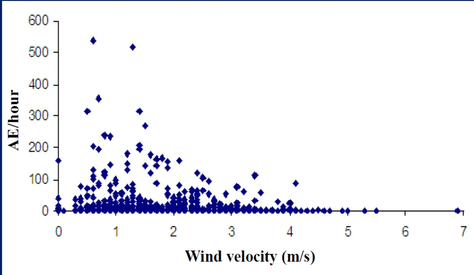
Chart relating the wind velocity and the AE count rate during all the monitoring period (2915 hours).
