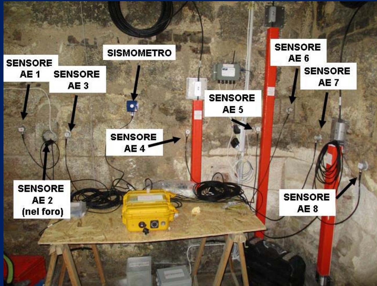
**Arrangement of the AE sensors inside the Garisenda Tower cell**
