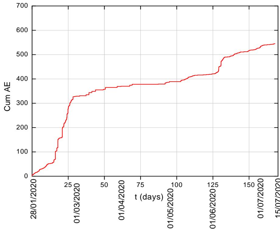
**AE cumulative count and wind velocity detected around the Garisenda Tower.**
