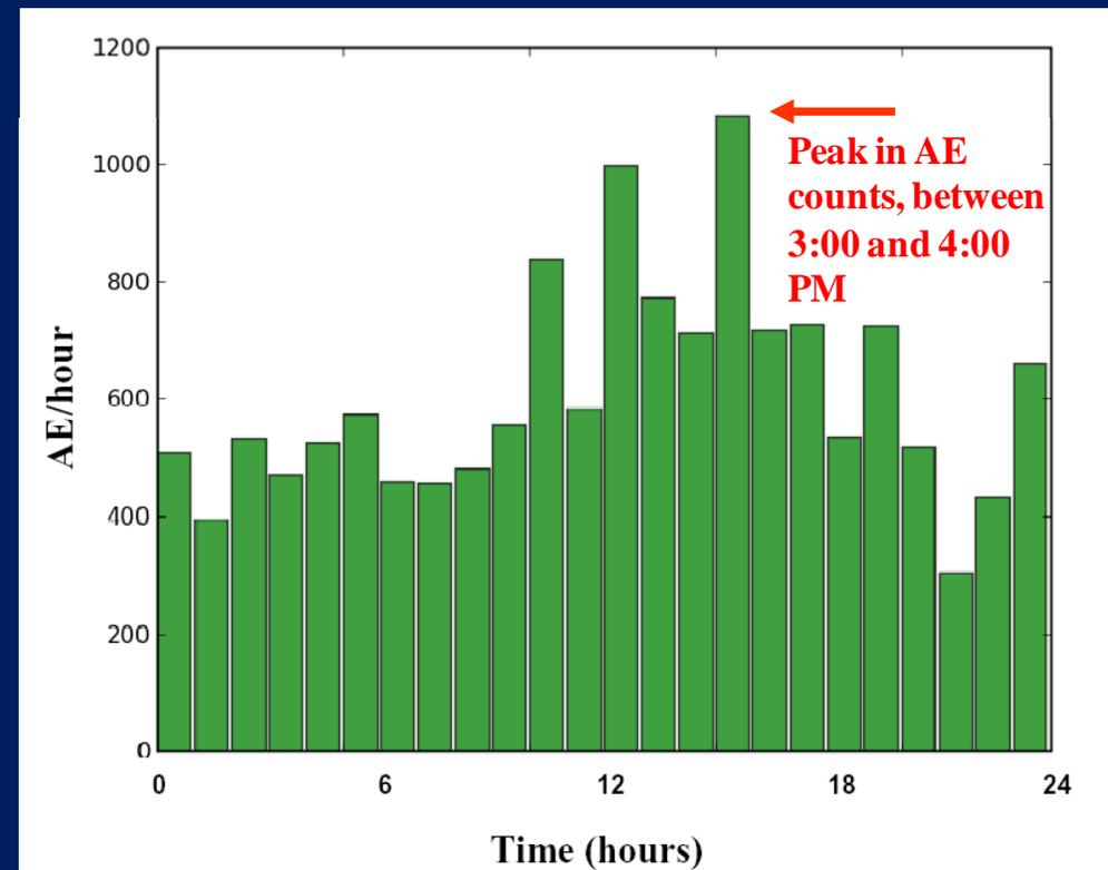
The comparison between the two distributions reveals as, during the monitoring period, the traffic effects on the damage to the tower were negligible.
