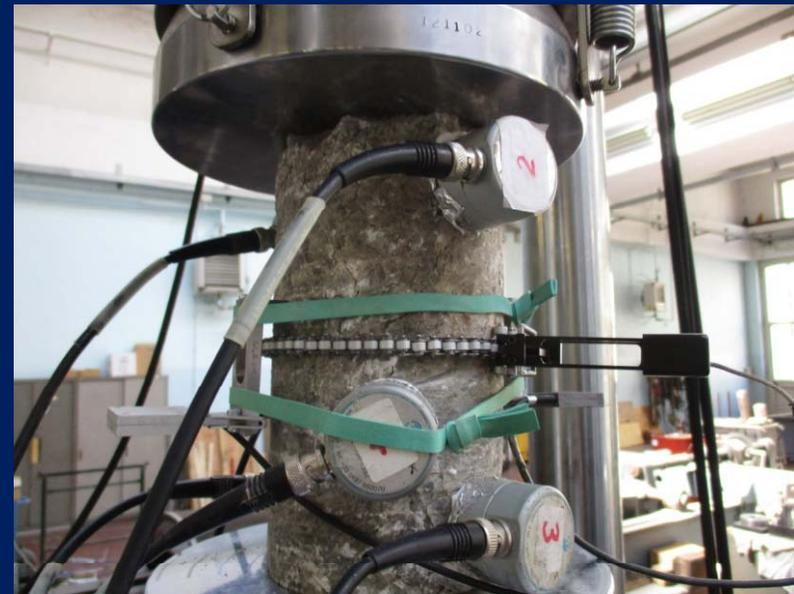
**Compression test on a specimen with slenderness 2.
