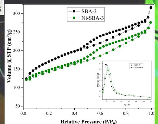
Adsorption-desorption isotherm and pores distribution
