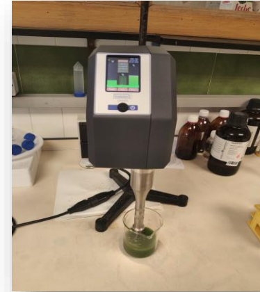
Sonotrode ultrasound assisted extraction
