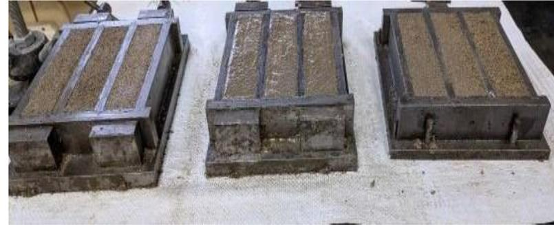
**RCxS** mortar from 20% per weight from **fine recycled concrete aggregates** see and 80% from **standard sand**
