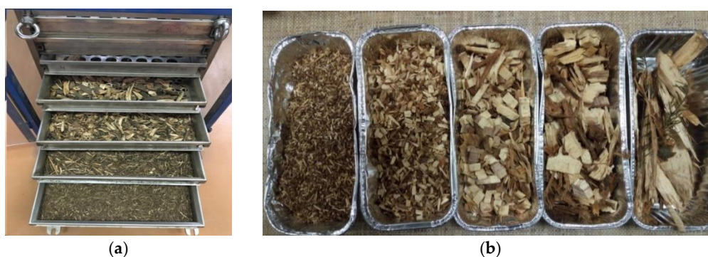
Figure 1. Łukomet separator and fractionated samples: (a) screen separator with round openings conforming to PN-ISO 565:2000 and PN-ISO 3310-2:2013; (b) pine chip size fractions.
