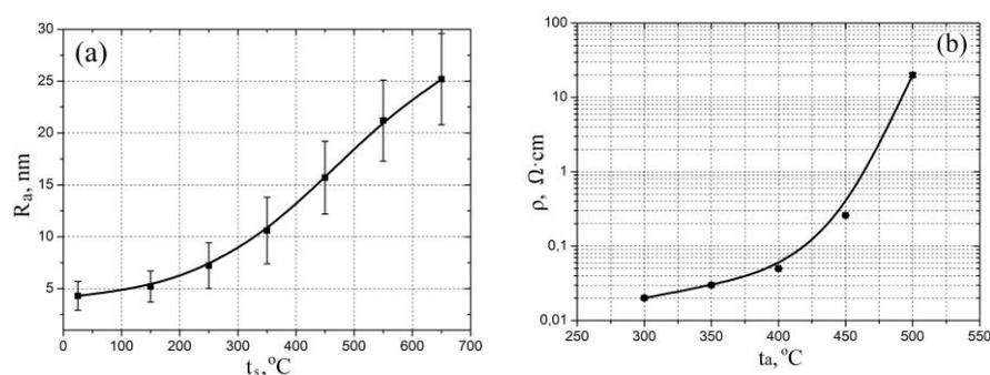
**Figure 2.** Dependence of the geometric and electrophysical parameters of a nanocrystalline vanadium oxide film on the control parameters of the PLD (a)—surface roughness on substrate temperature; (b)—resistivity on annealing temperature.
