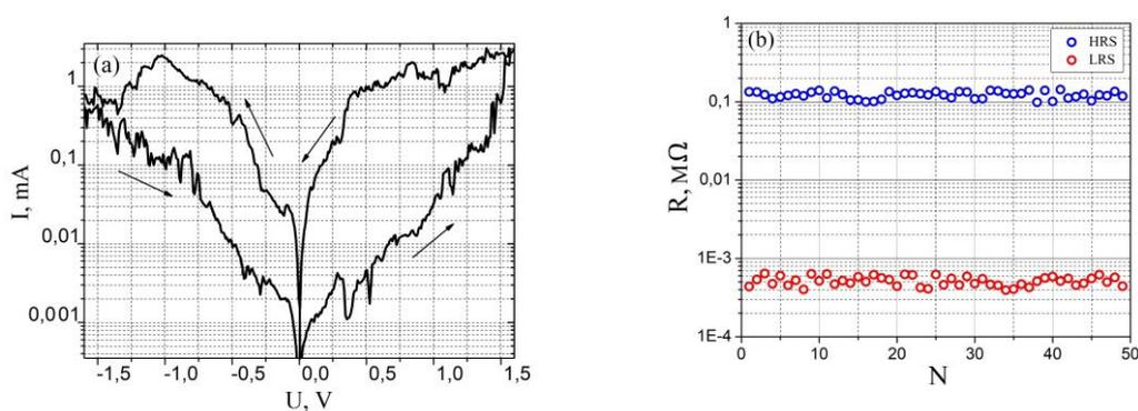
**Figure 3.** Investigation of resistive switching effect in nanocrystalline vanadium oxide film (a)—current-voltage characteristics; (b)—endurance test.
