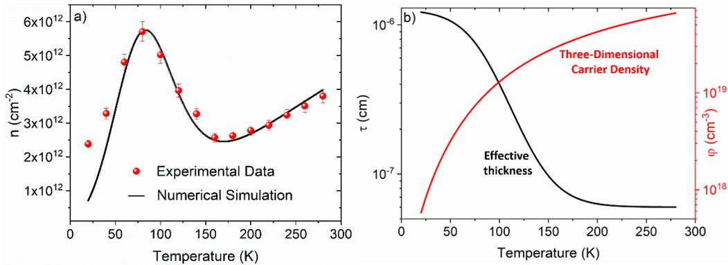
**Figure 3.** (a) Numerical simulation of the 2D carrier density as function of the temperature for  $V_{gs} = -20 \text{ V}$  superimposed to the experimental data (red dots). (b) Effective thickness of the channel (black line) and three-dimensional carrier density (red line) as function of the temperature for  $V_{gs} = -20 \text{ V}$
