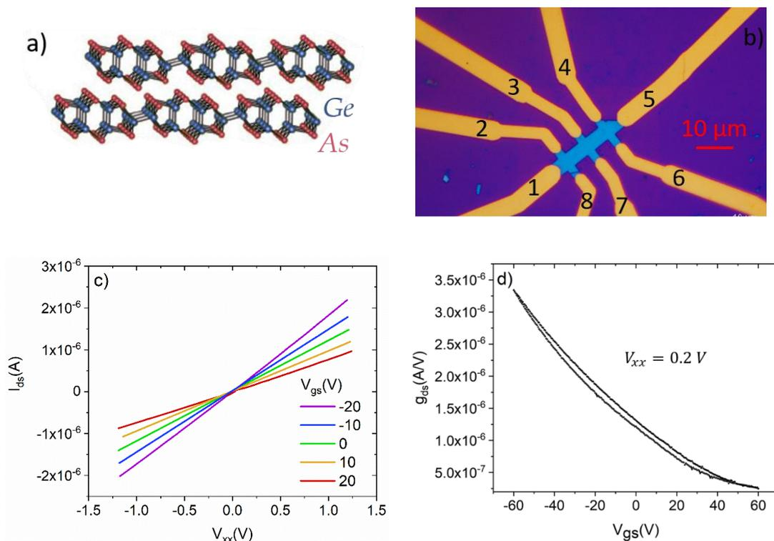
**Figure 1.** (a) Atom arrangement in *GeAs* layers. (b) Optical image of the Hall bar device with *Ni/Au* electrodes. (c) Output characteristic recorded in four-probe configuration with  $V_{gs}$  bias between  $-20$  V and  $20$  V. (d) Transfer characteristic recorded in four-probe configuration showed both on linear and logarithmic scale.
