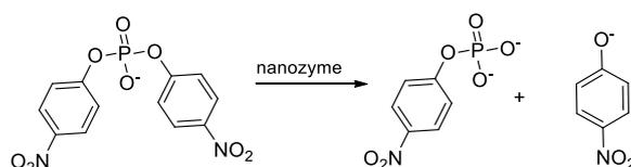
**Figure 2.** Hydrolysis of BNP by gold nanozymes.
