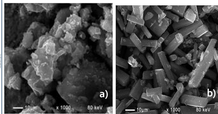
Figure 3. SEM images of lead citrate precursor synthesized by desulfurization and leaching of: a) a used PAM; b) a mixture of used PAM and NAM.
