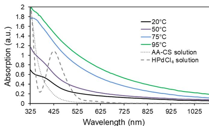
**Figure 1.** The UV-Vis absorption spectra of AA-CS solution,  $\text{HPdCl}_4$  solution, and PdNPs solutions from four different temperature synthesis conditions.
