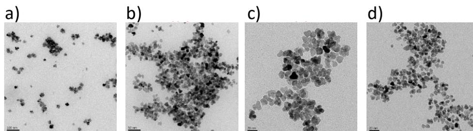
**Figure 2.** TEM images of PdNPs from four experiments: (a) 20 °C, (b) 50 °C, (c) 75 °C, and (d) 95 °C.
