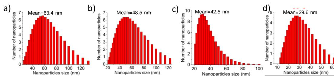
**Figure 3.** Size distribution of PdNPs from four experiments: (a) 20 °C, (b) 50 °C, (c) 75 °C, and (d) 95 °C.
