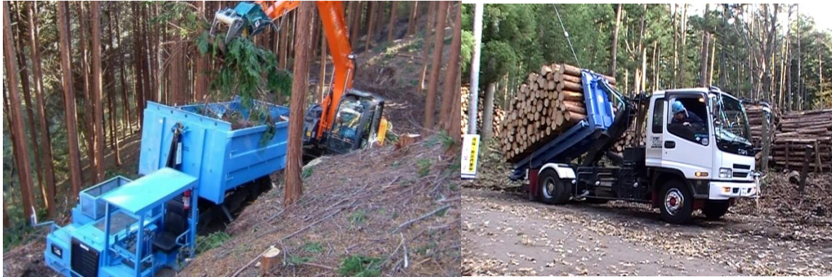
Figure 5. An arm roll forwarder with 3-m logs (Top left), 2-m logs (Top right), and biomass containers (Bottom left), and an arm roll truck (Bottom right).
