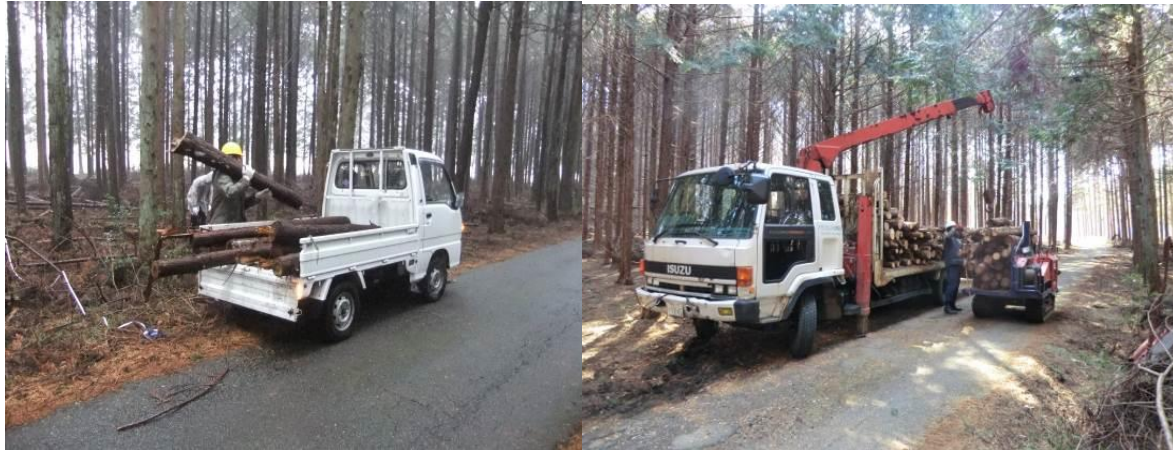
Figure 1. Loading to a light truck by individual forest owners (Left) and unloading from mini-forwarder with truck crane by a private logging contractor (Right).
