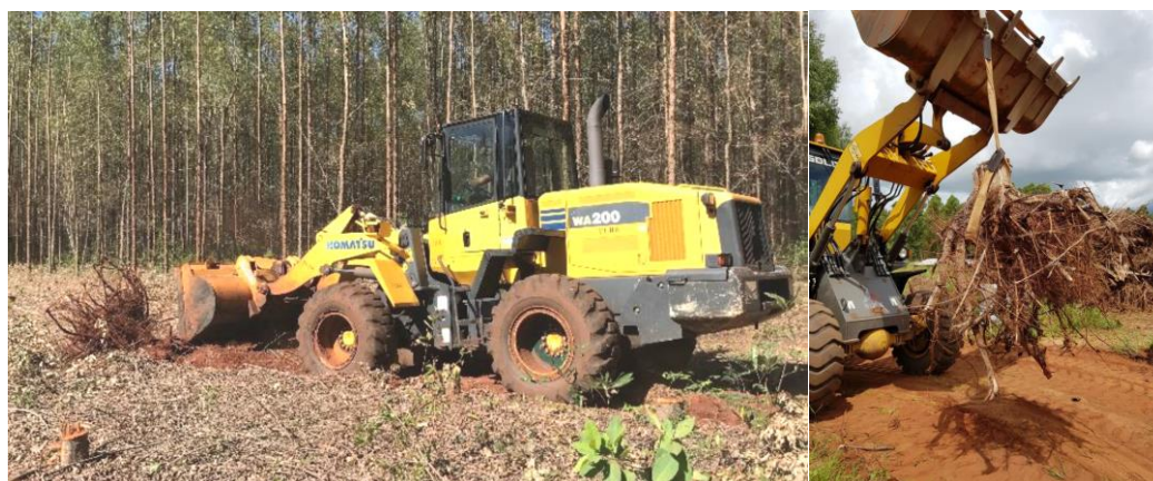
Figure 1. Stumps pulled off the ground and weighted with a portable dynamometer.
