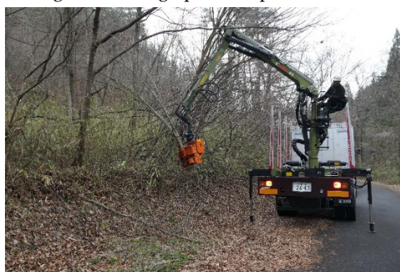
Figure 2. Harvesting experiment with a truck-mounted multi-tree felling head.
