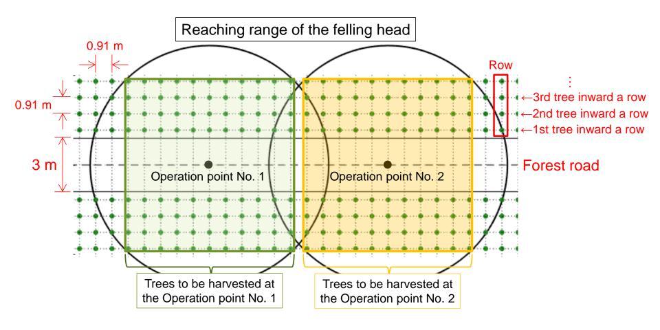
When a felling machine harvested the coppice trees repeatedly with moving each operation point in turn, the number of felled trees inward a row that minimized the harvesting cost was examined.
