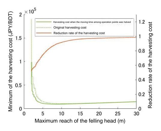
The following future policy for the machine's improvement was suggested: Raising the moving velocity of a felling head and increasing the maximum number of trees that can be held at a time are effective if lengthening the maximum reach of a felling head is possible. In the meantime, shortening the machine's moving time among operation points is effective unless the maximum reach of a felling head is lengthened.
