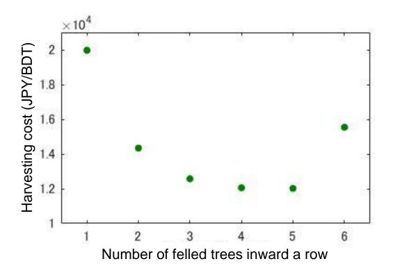
The more trees inward a row the machine felled, the more trees were harvested at one operation point. In this case, however, the machine's total moving time markedly increased because the frequency of moving among operation points increased. Therefore, it was concluded that there was the optimum number of felled trees inward a row that could minimize the harvesting cost.
