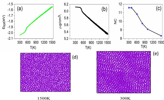
**Fig.2** (a) Total energy per atom, (b) density, (c) coordination number ( $N_c$ ), (d) structure of liquid tellurium (Te) at 1500 K, and (e) 300 K during solidification process at distinct temperatures
