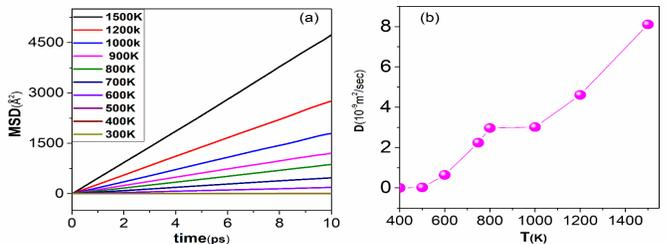
**Fig.5** (a) The mean square displacement (MSD) with time dependence, and (b) variation of the self-diffusion coefficient at distinct temperatures during the cooling process.
