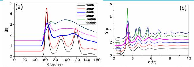
**Fig.3** (a) Bond-angle distribution functions, and (b) structure factor of liquid tellurium (Te) at distinct temperatures.
