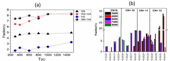
**Fig.4** (a) Fractions percent of pair analysis, and (b) top voronoi-index clusters of liquid tellurium (Te) at distinct temperatures during the solidification process.
