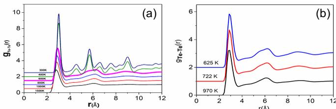
**Fig.1** (a,b) Radial distribution function of liquid tellurium (Te) during solidification process.
