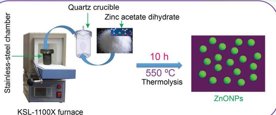
Figure 1: The synthesis process of ZnO-NPs from Zinc acetate dihydrate by thermal method.
