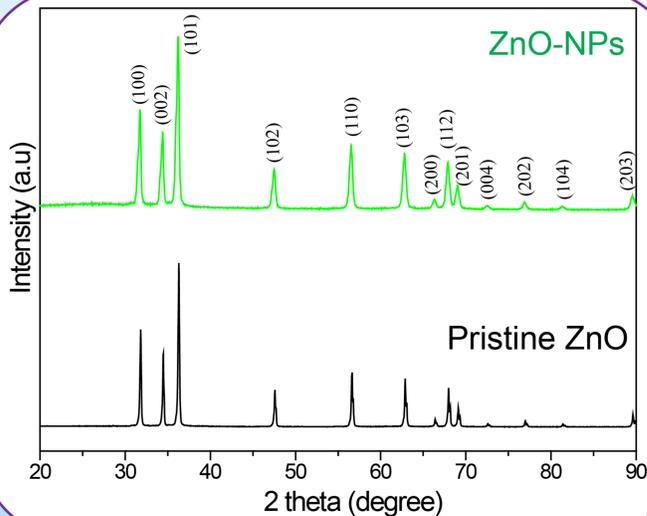
Figure 2: XRD patterns of the synthesized ZnO-NPs, and pristine ZnO.
