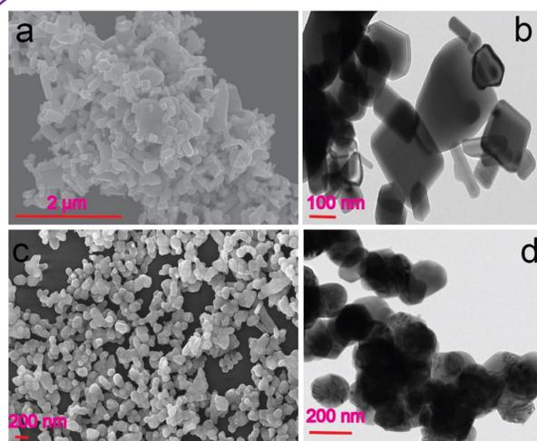
Figure 3: (a), (c) FE-SEM of Pristine ZnO and synthesized ZnO-NPs; (b), (d) TEM of Pristine ZnO and synthesized ZnO-NPs.
