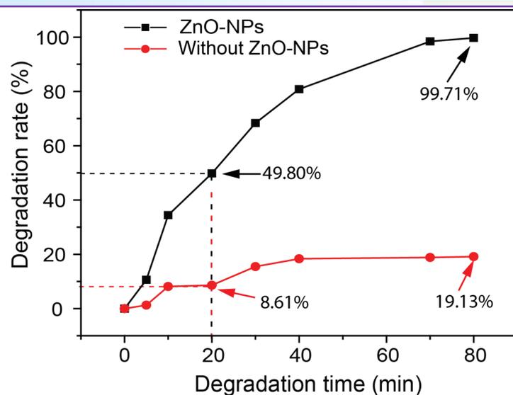
Figure 5: Photocatalytic degradation of synthesized ZnO-NPs, and without ZnO-NPs.
