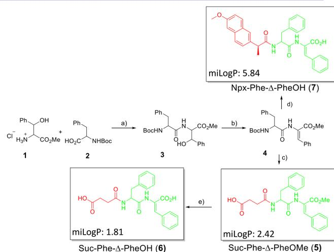
**Figure 1:** General methodology for the synthesis of dehydrodipeptides: a) HBTU, TEA, MeCN; b) i. Boc<sub>2</sub>O/DMAP, MeCN, ii. TMG; c) i. TFA, ii. anhydride succinic, pyridine; d) i. TFA, ii. Naproxen chloride, TEA; e) NaOH 1M; dioxane.
