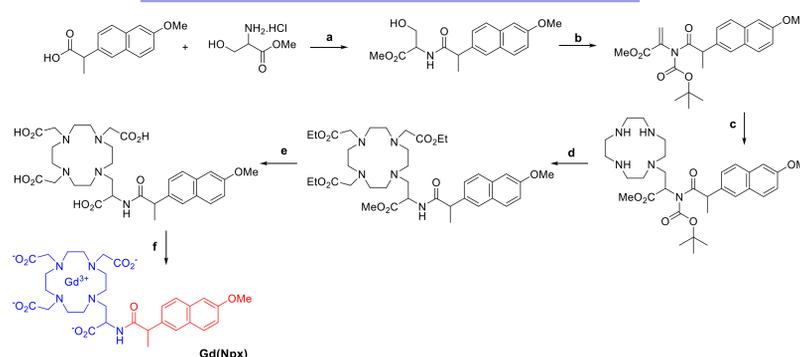
**Figure 2.** Synthetic pathway for the synthesis of the Gd(Npx) complex: a) DCC/HOBT, TEA, DCM; b) Boc<sub>2</sub>O/DMAP, MeCN; c) Cyclen, K<sub>2</sub>CO<sub>3</sub>/MeCN; d) i. TFA/DCM; ii. K<sub>2</sub>CO<sub>3</sub>, MeCN; iii. ethyl bromoacetate; e) i. Dowex-1X2-OH<sup>-</sup> H<sub>2</sub>O/EtOH; ii. elution with HCl (0,1M); f) GdCl<sub>3</sub>.
