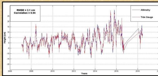
Figure 4: Altimetric data vs tide gauge data
