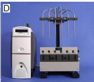
Parts of the  $\mu$ DISS profiler system. A) Steel dies with compressed powder. B) Dies inserted into teflon rotating disk carriers. C) Rotating disk carriers with dies placed on the bottom of the glass vials. Fibre optic probes are immersed into dissolution medium. D)  $\mu$ DISS Profiler. (Pictures from avdeef and Tsinman 2008)
