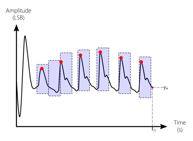
PPG – HR and BR. Local maxima finding Adaptive filtering Unstable signals rejection Frequency extraction
