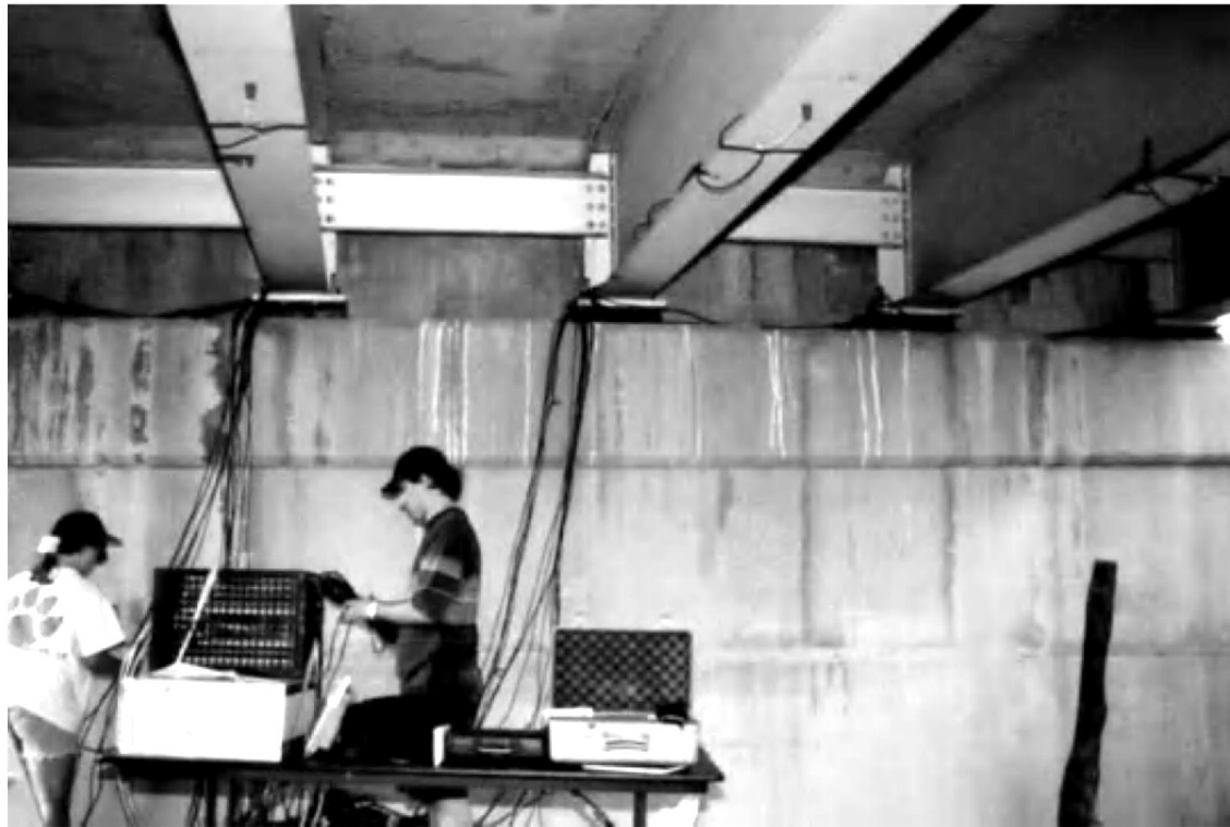
Bridge sensor acquisition system (from "Structural Health Monitoring" C.R. Farrar, K. Worden)
