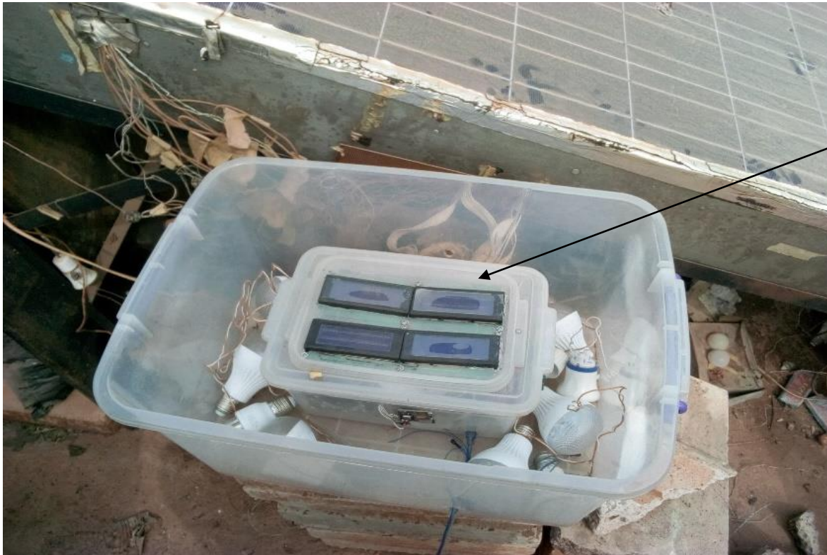
Fig. 2 the temperature data logger displaying values of Temperatures.
