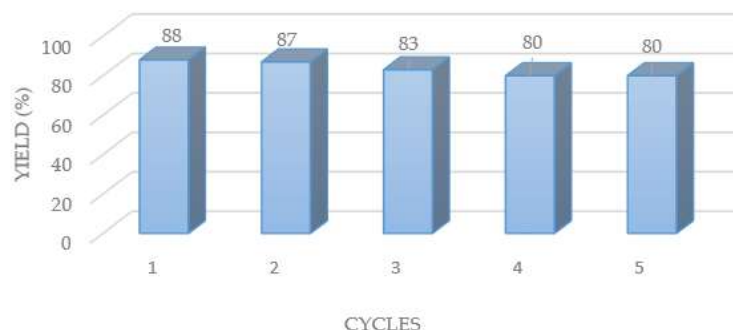
Figure 3. Recyclability of the PdNPs/BC catalyst in the direct synthesis of carbazole 3 .
