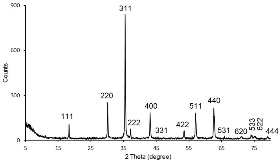
**Figure 2.** XRD pattern of  $\text{CoFe}_2\text{O}_4$ .
