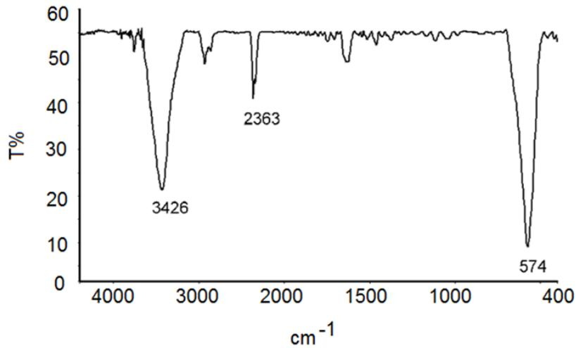
**Figure 1.** FT-IR spectrum of the prepared  $\text{CoFe}_2\text{O}_4$ .
