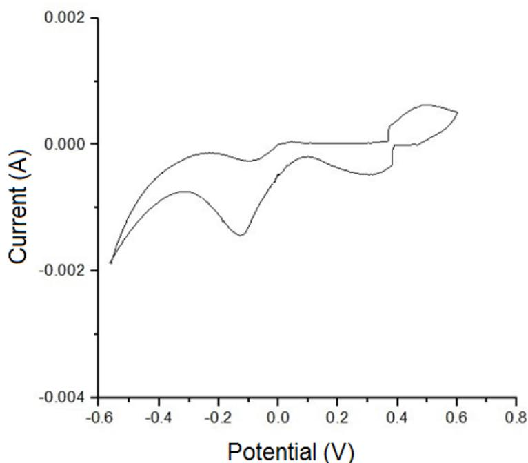
**Figure 5.** CV curves of the product at the potential scan rate of 10 mVs<sup>-1</sup>.
