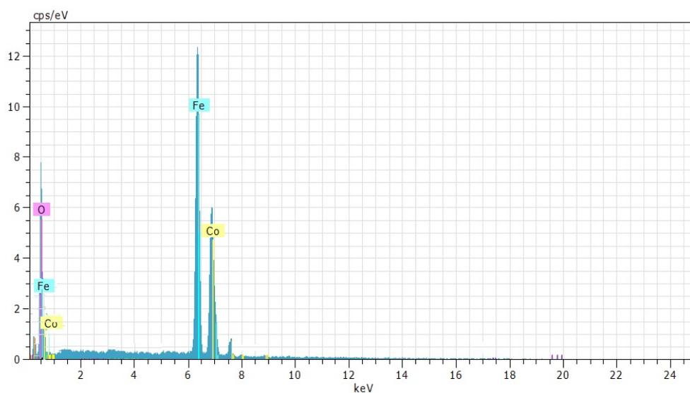
**Figure 3.** EDX analysis of the resulting cobalt ferrite.
