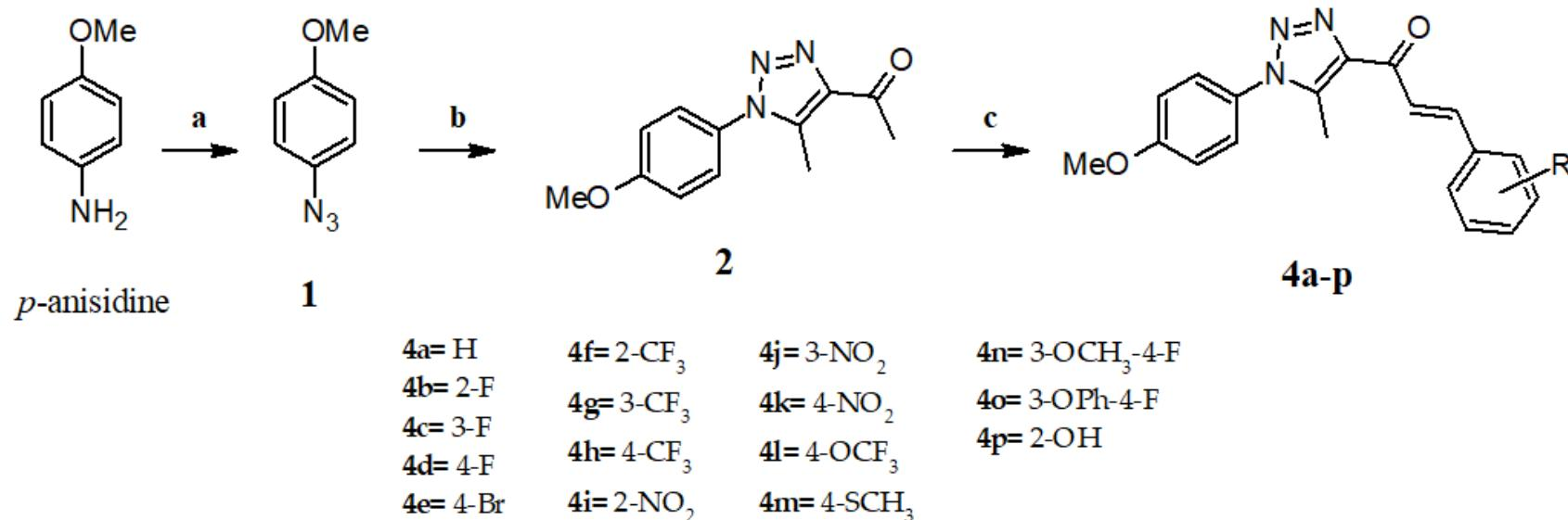
Reagents and conditions: (a) i. KHSO<sub>4</sub>, ii. NaNO<sub>2</sub>, iii. NaN<sub>3</sub>, r.t., (b) acetylacetone, K<sub>2</sub>CO<sub>3</sub>, DMSO, r.t., (c) Benzaldehyde **3a-p**, KOH, EtOH, 0°C, 2h → rt.
