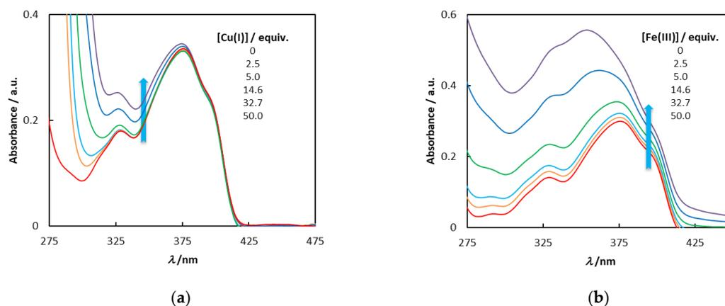
**Figure 2.** Absorption spectra of **1** ( $5.0 \times 10^{-6}$  M in  $\text{CH}_3\text{CN}:\text{CHCl}_3$  (1:1)) upon addition of increasing amounts of (a)  $\text{CuOAc}$  and (b)  $\text{Fe}(\text{ClO}_4)_3$  ( $1.24 \times 10^{-5}$ – $2.50 \times 10^{-4}$  M).
