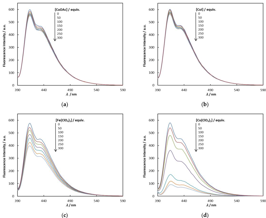
**Figure 1.** Emission spectra of **1** ( $1.0 \times 10^{-7}$  M in  $\text{CH}_3\text{CN}:\text{CHCl}_3$  (1:1)) upon addition of increasing amounts (up to 300 equiv.) of CuOAc (a), CuI (b),  $\text{Fe}(\text{ClO}_4)_3$  (c) and  $\text{Cu}(\text{ClO}_4)_2$  (d) ( $\lambda_{\text{exc}} = 380$  nm).
