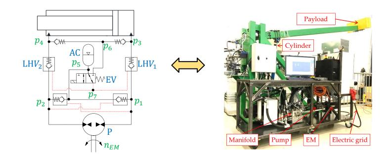
\* Padovani et al.: "A Self-Contained Electro-Hydraulic Cylinder with Passive Load-Holding Capability," 2019.
