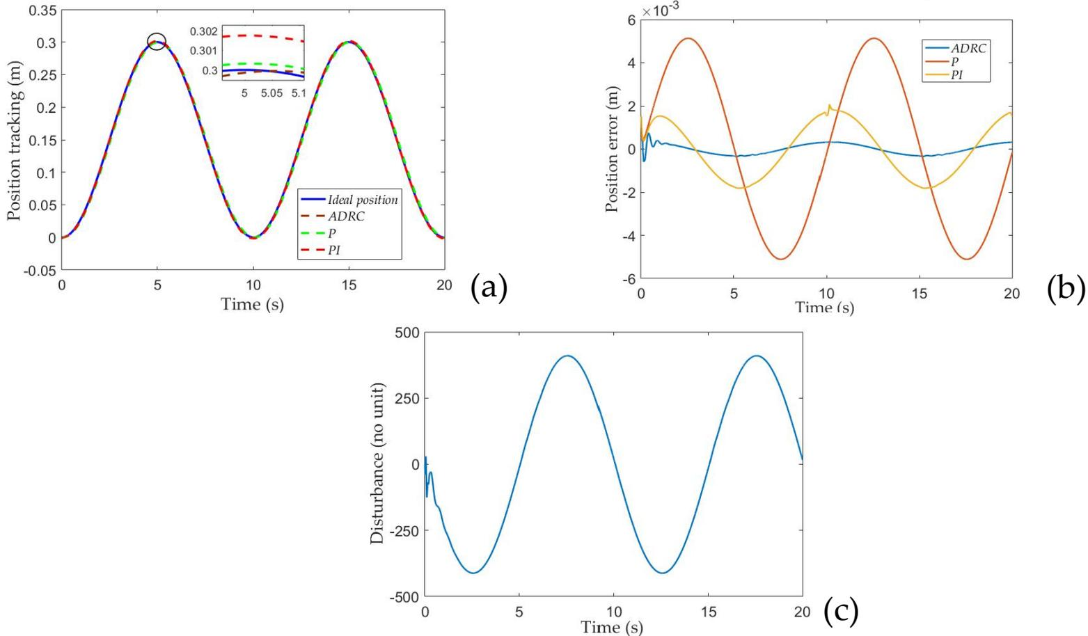
**Figure 5.** The sine position signal tracking without disturbance: (a) position tracking ; (b) position tracking error ; (c) total disturbance observation.
