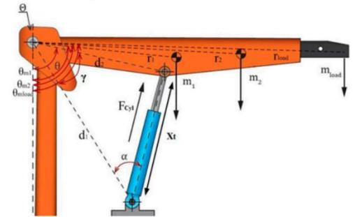
Figure 2. Crane structure diagram [8]
