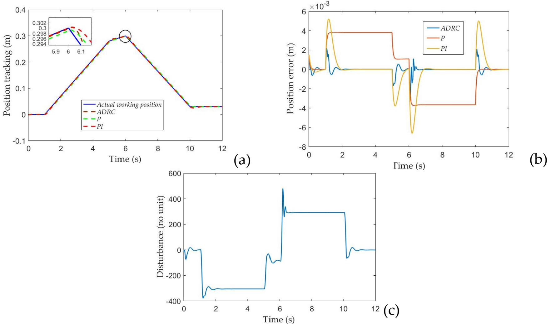
**Figure 7.** The actual working position signal tracking without disturbance: (a) position tracking ; (b) position tracking error ; (c) total disturbance observation.
