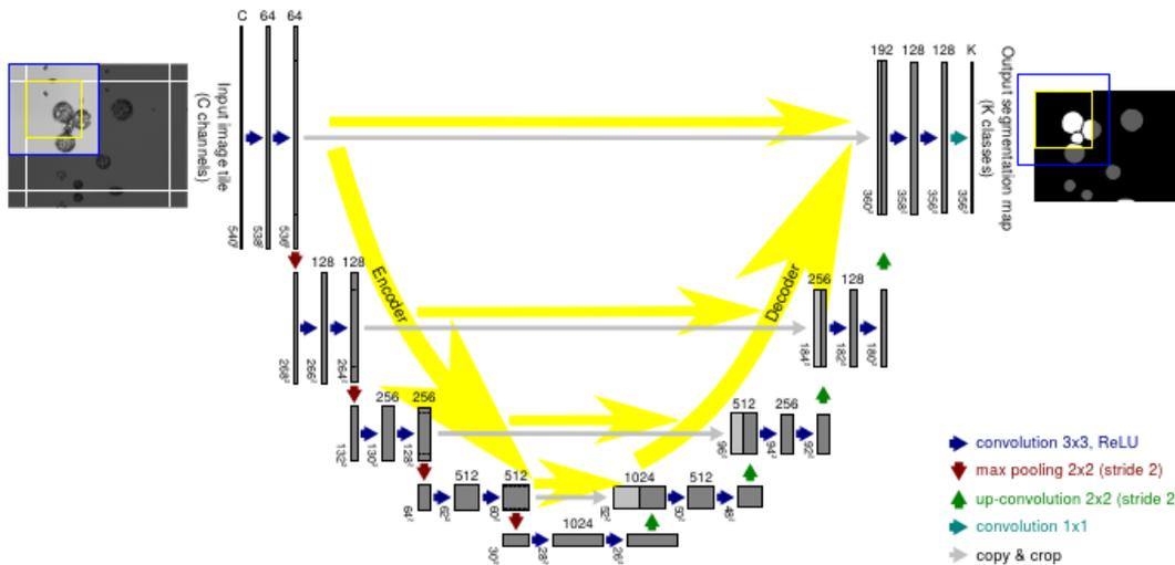
Figure 2. Architecture of U-Net [12].
