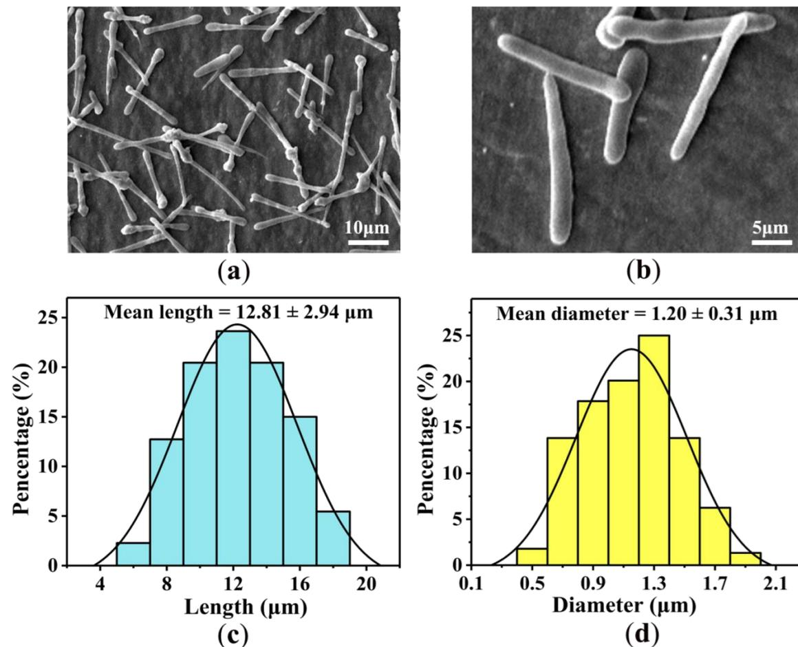
**Figure 2.** SEM images of  $\text{Fe}_3\text{O}_4/\text{NaYF}_4: \text{Eu}^{3+}/\text{PLGA}$  microrods at different magnifications, (a)  $\times 5000$ , (b)  $\times 10000$ ; (c) length distribution and (d) diameter distribution of  $\text{Fe}_3\text{O}_4/\text{NaYF}_4: \text{Eu}^{3+}/\text{PLGA}$  microrods.
