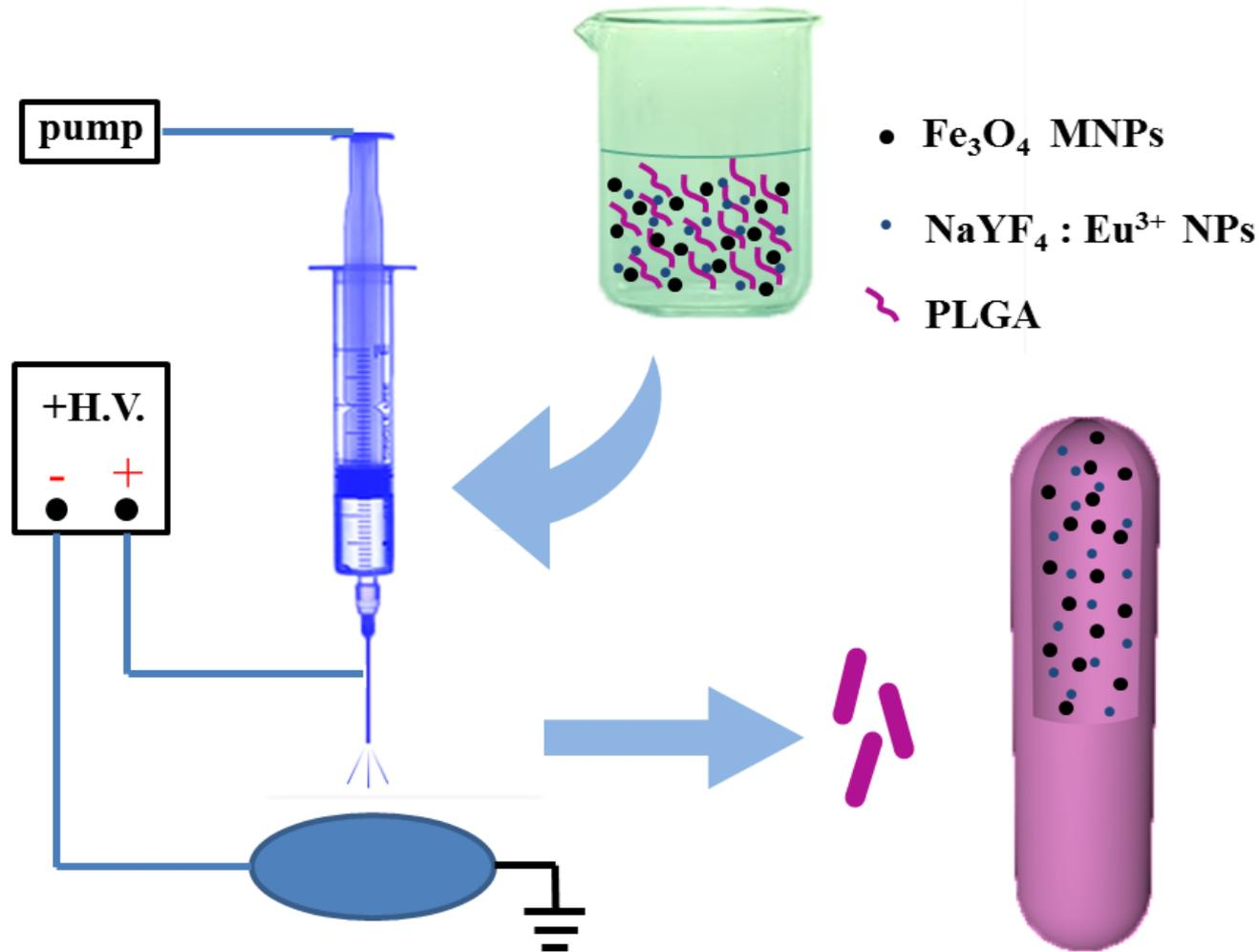
**Figure 1.** Schematic illustration of the preparation of the  $\text{Fe}_3\text{O}_4/\text{NaYF}_4:\text{Eu}^{3+}/\text{PLGA}$  magnetic-fluorescent bifunctional microrods.
