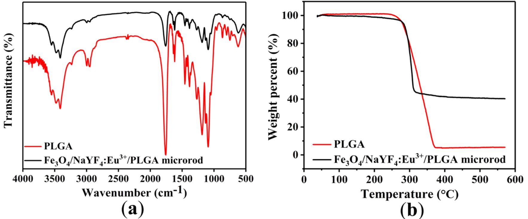
**Figure 3.** (a) FTIR spectra of PLGA and Fe<sub>3</sub>O<sub>4</sub>/NaYF<sub>4</sub>:Eu<sup>3+</sup>/PLGA microrods; (b) TG curve of PLGA and Fe<sub>3</sub>O<sub>4</sub>/NaYF<sub>4</sub>:Eu<sup>3+</sup>/PLGA microrods.
