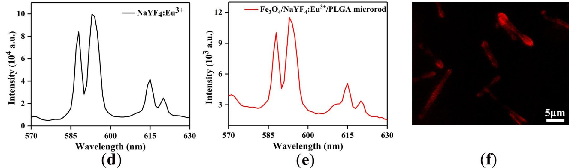
**Figure 4.** Emission spectra of (d) pure  $\text{NaYF}_4:\text{Eu}^{3+}$  NPs and (e)  $\text{Fe}_3\text{O}_4/\text{NaYF}_4:\text{Eu}^{3+}/\text{PLGA}$  microrods. (f) Fluorescent photograph of the  $\text{Fe}_3\text{O}_4/\text{NaYF}_4:\text{Eu}^{3+}/\text{PLGA}$  microrods.
