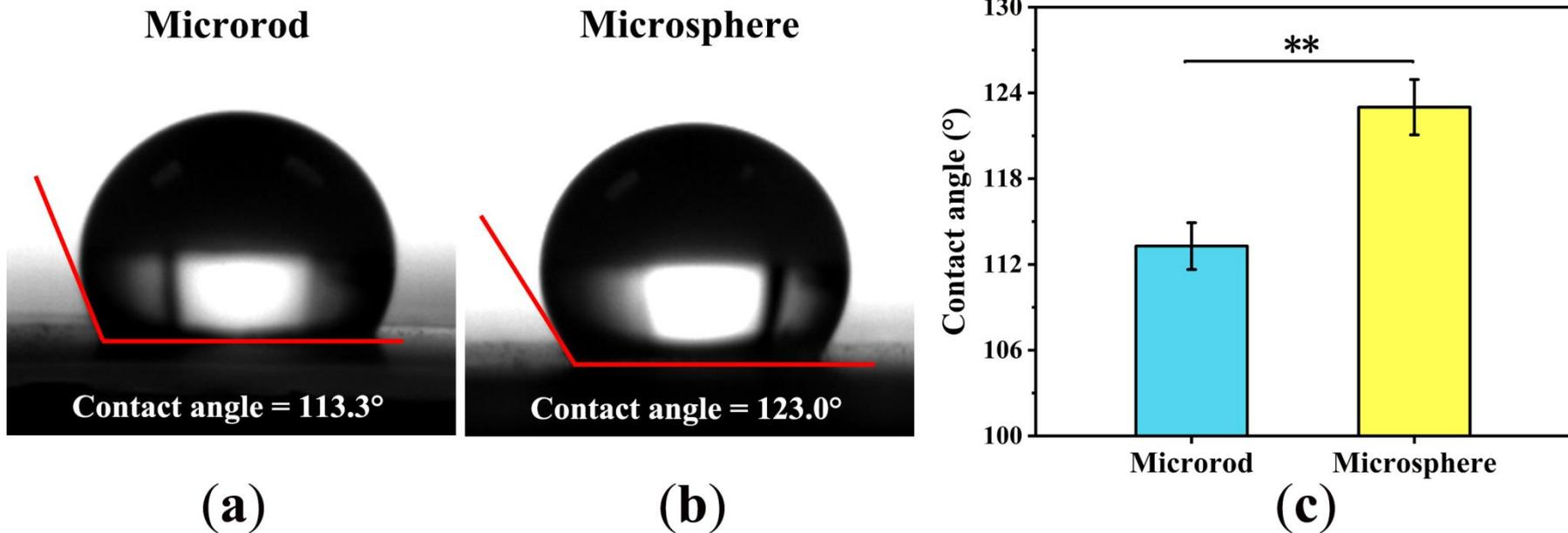
**Figure 5.** Images of water droplets on (a)  $\text{Fe}_3\text{O}_4/\text{NaYF}_4:\text{Eu}^{3+}/\text{PLGA}$  microrods and (b)  $\text{Fe}_3\text{O}_4/\text{NaYF}_4:\text{Eu}^{3+}/\text{PLGA}$  microspheres; (c) contact angles and of  $\text{Fe}_3\text{O}_4/\text{NaYF}_4:\text{Eu}^{3+}/\text{PLGA}$  microrods and microspheres,  $n=3$ .
