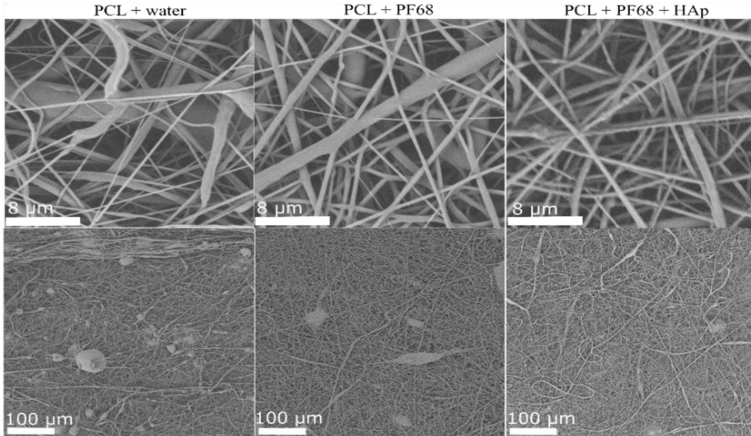
Fibres made with HAp appear to be more rough, clusters of HAp can also be observed showing that HAp was successfully incorporated. Moreover, the improvement in morphology is clearly visible in from PCL+water to PCL+PF68+HAp, where the best morphology was obtained with incorporated HAp.
