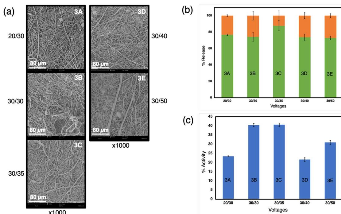
**Figure 3.** The influence of different voltages (3A-20/30, 3B-30/30, 3C-30/35, 3D-30/40, 3E-30/50) on (a) the morphology of fibers; (b) HRP burst release from scaffolds; (c) HRP activity.
