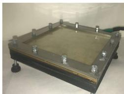
Figure 1. Laboratory-developed cast-moulding device.
