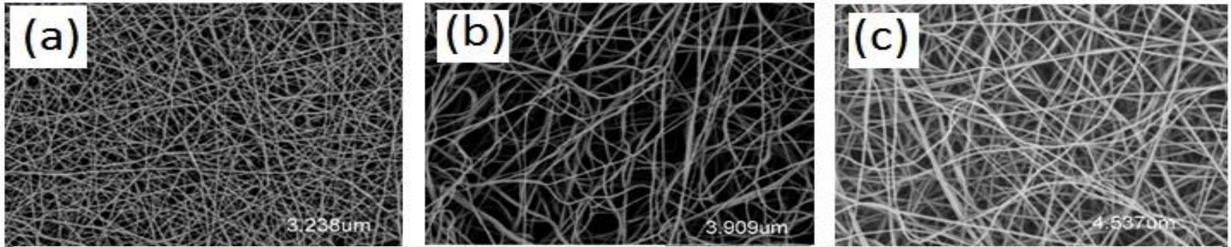
Scanning electron microscopy (SEM) images of (a) blank PVA nanofibers, BNF0 formulation, (b) gliclazide nanofibers, GLZNF1 formulation, and (c) optimized gliclazide nanofibers, GLZNF2 formulation.
