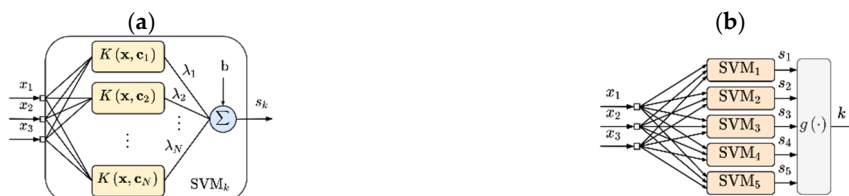
Figure 2. Schematic representation of SVM (a) models used for classification of physical the samples of nanocarriers.
