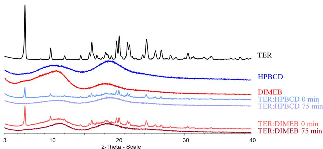
**Figure 1.** XRPD diffractograms of TER and products.
