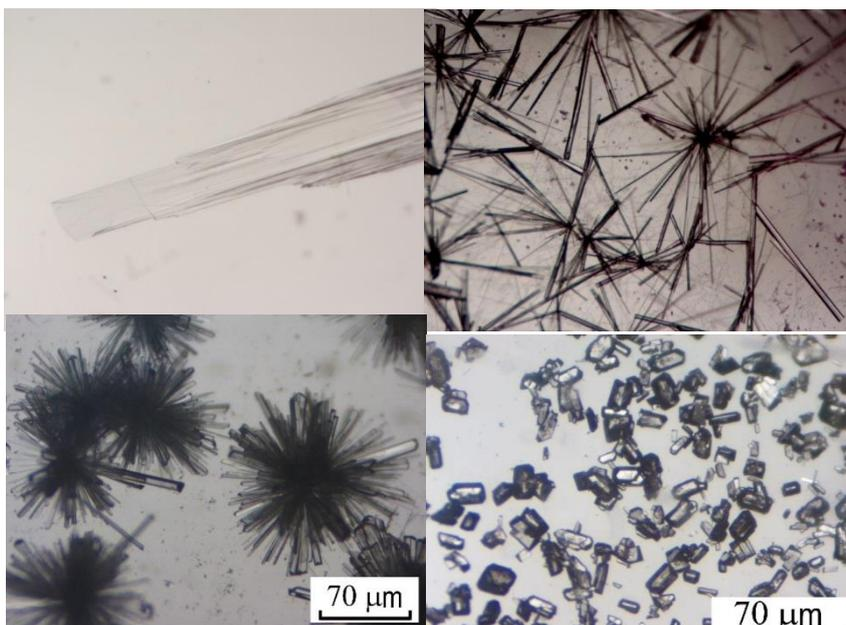
Figure 3, Top, DIF/EBIPy crystallised without additive (left) and with SPY (right).
