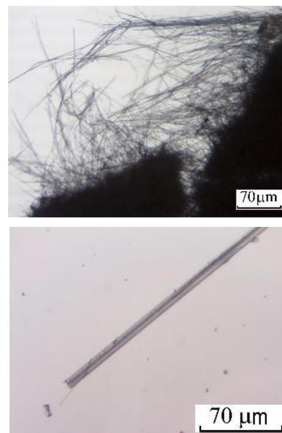
Figure 2, DIF/INA crystallised from the gas phase without (top) and with the presence of benzamide (Bottom. Reproduced from [17] with permission from the Royal Society of Chemistry
