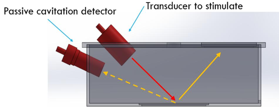
1 MHz transducer to stimulate; 7.5 MHz transducer to record
