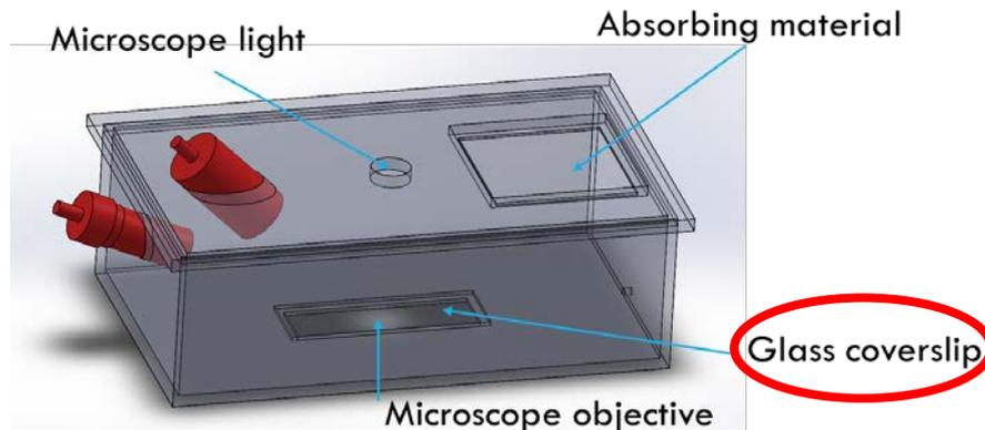
Microscope-compatible water tank (190x110x60 mm)
