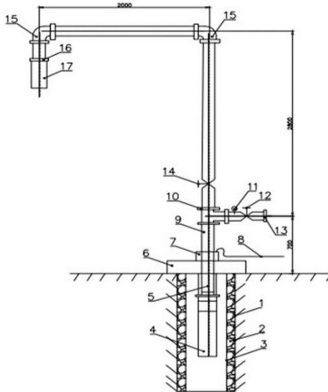
Figure 1. The proposed support point for fire water supply
