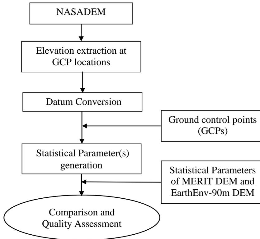
**Figure 2:** Flowchart for Quality Assessment of openly accessible NASADEM products with GCPs and its comparison with MERIT DEM and EarthEnv 90m DEM [8], [9]
