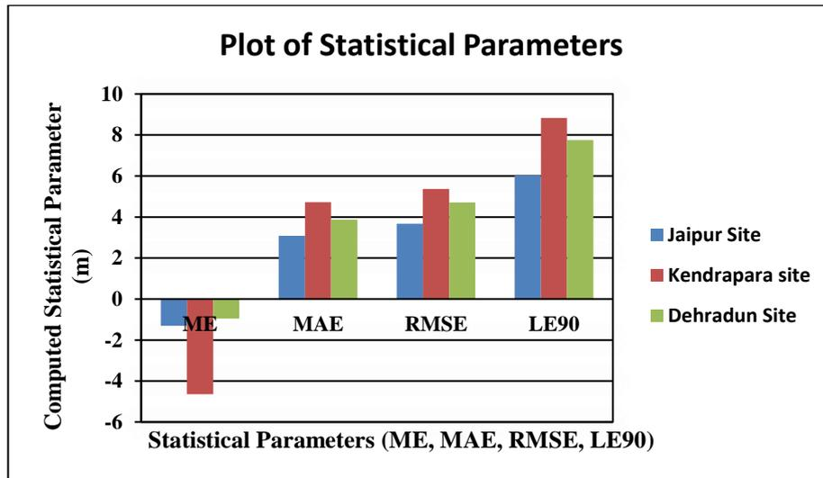
Figure 6: Plot of ME, MAE, RMSE and LE90 for NASADEM datasets at three experimental sites
