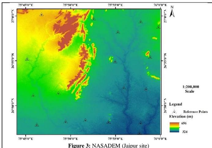
*vertical accuracy and the statistical parameters, such as mean error (ME), mean absolute error (MAE), and root mean square error (RMSE). The RMSE of 4.71m at the Dehradun site depicts that in undulating regions NASADEM is performing better than both EarthEnv-DEM90 and MERIT DEM. However, in the case of urban and plain regions, the performance of MERIT DEM and EarthEnv DEM is superior to that of NASADEM.*
