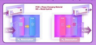
The tank is based on an innovative concept that couples hydrogen and heat storage for stationary storage of the excess renewable energy.
