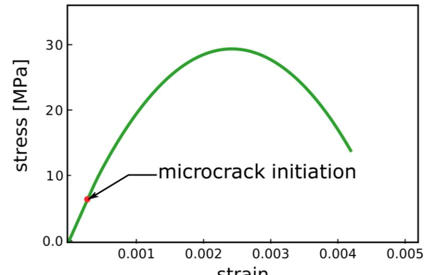
Homogenized concrete behaviour in uniaxial compression
