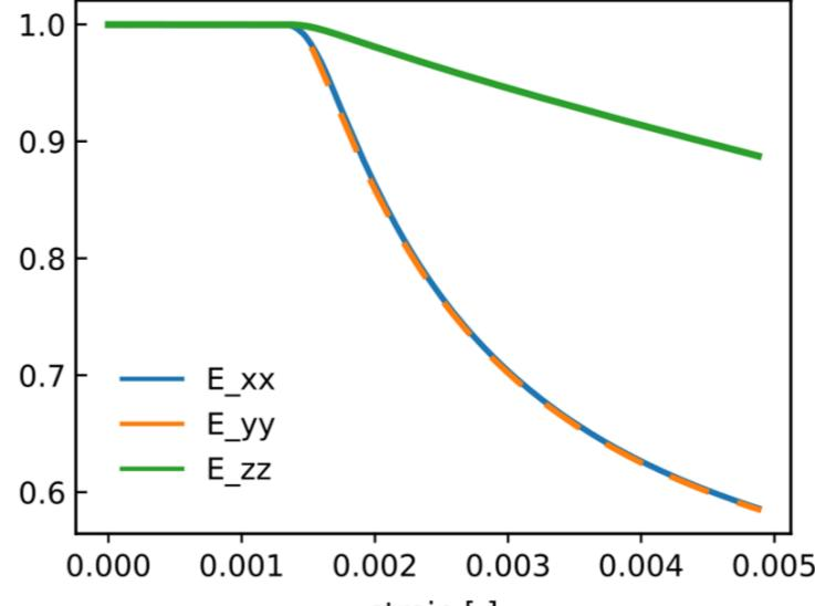
Concrete stiffness reduction in uniaxial compression
