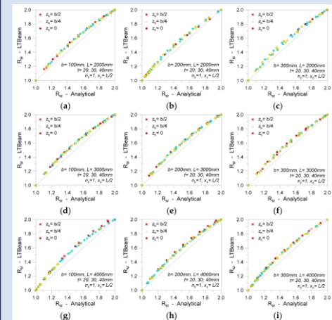
4. Normalized comparative LTB calculations for LR glass beams with mechanical point fixings variably positioned on the span and with variable local restraining stiffness  $K_b$ . Reproduced from [1] under the terms and conditions of CC BY license
