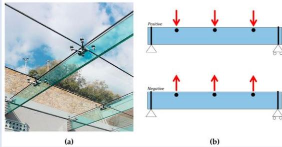
1. Typical example of (a) laterally restrained (LR) glass beams with discrete mechanical restraints and (b) schematic representation of the reference loading configurations for LR beams in LTB (associated, in the order, to positive or negative bending effects). Reproduced from [1] under the terms and conditions of CC BY license
