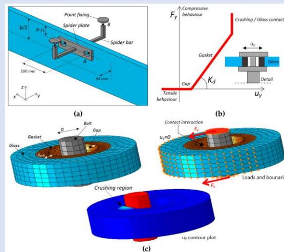
3. FE numerical modeling of a glass beam with LR in LTB ( $n_b = 1, x_b = L/2$ ): (a) geometrical detail of the mechanical (spider) restraint, with evidence of (b) the proposed mechanical characterization of gaskets (detail "B" from (a)). In (c), an example is proposed in the form of local FE numerical model for the LR stiffness characterization and analysis of a "detail B" point-fixing (ABAQUS/Standard). All the figures are reproduced from [1] under the terms and conditions of CC BY license
