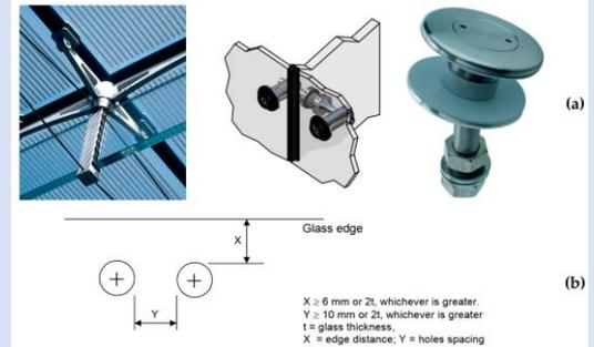
2. Detail of LR glass beams with discrete mechanical lateral restraints: (a) examples of point fixings and (b) schematic representation of minimum distance requirements for the glass holes. Reproduced from [1] under the terms and conditions of CC BY license
