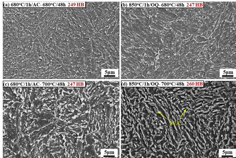
Figure 5. Microstructure of sample austenitized and then annealing: (a) 680°C/1h/AC-680°C/48h, (b) 850°C/1h/OQ-680°C/48h, (c) 680°C/1h/AC-700°C/48h, (d) 850°C/1h/OQ-700°C/48h.
