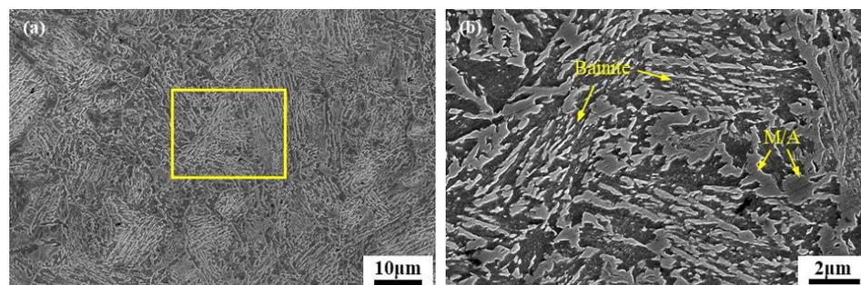
Figure 1. (a) SEM micrographs of hot-rolled sample; (b) Enlarged image of the yellow square in (a).
