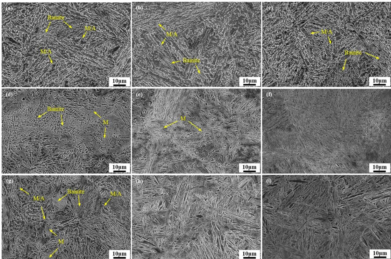
**Figure 2.** SEM micrographs of different initial microstructures obtained by different austenitizing process. (a) 680 °C/1h/AC; (b) 680 °C /1h/OQ; (c) 680 °C/1h/WQ; (d) 850 °C/1h/AC; (e) 850 °C/1h/OQ; (f) 850 °C/1h/WQ; (g) 1000 °C/1h/AC; (h) 1000 °C/1h/OQ; (i) 1000 °C/1h/WQ.
