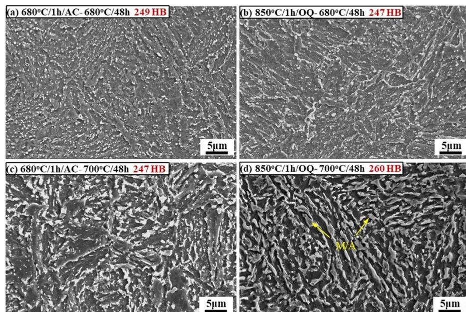
Figure 5. Microstructure of sample austenitized and then annealing: (a) 680°C/1h/AC-680°C/48h, (b) 850°C/1h/AC-680°C/48h, (c) 680°C/1h/AC-700°C/48h, (d) 850°C/1h/AC-680°C/48h.
