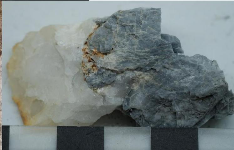
To date, pegmatite dykes comprising a main assemblage of quartz-microcline-orthoclase-(labradorite-andesine-albite) have been found on levels 285, 310 and 615. They have hypidiomorphic granular textures and in places contain cavities lined with later chlorite, siderite, stilbite-Ca and pyrite.
